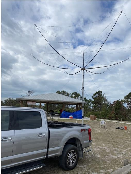
5 band hex beam on N4LJT truck bumper mount and push up pole
